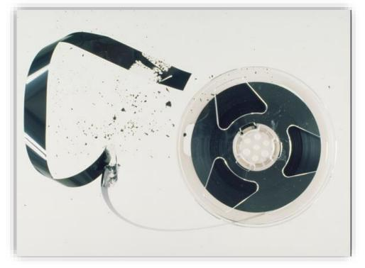
**Vinegar Syndrome:** Vinegar syndrome is a concern for acetate-based tape. More properly referred to as acetate film base degradation, vinegar syndrome is a very similar problem to nitrate base deterioration. Its causes are inherent in the chemical nature of the plastic and its progress very much depends on storage conditions.
