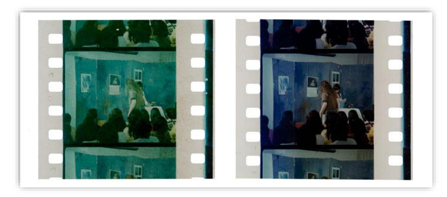
**Silver Fading:** Images on black and white film are typically formed by metallic silver in a gelatin binder. When exposed to a combination of moisture in the environment and pollutants in the air or contaminants in the film's enclosure, this image silver will corrode.
