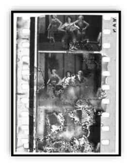
**Shrinkage:** Shrinkage is the loss of the original dimensionality of the film. Acetate and nitrate bases are both susceptible to a small initial amount of shrinkage after their manufacture due to the loss of solvents.
