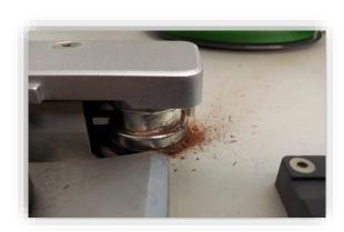
**Binder Degradation:** The binder is responsible for holding the magnetic particles on the tape and facilitating tape transport. If the binder loses integrity – through softening, embrittlement, loss of cohesiveness, or loss of lubrication – the tape may become unplayable. Sticky tape and sticky shed are commonly used terms to describe the phenomenon associated with deterioration of the magnetic tape binder
