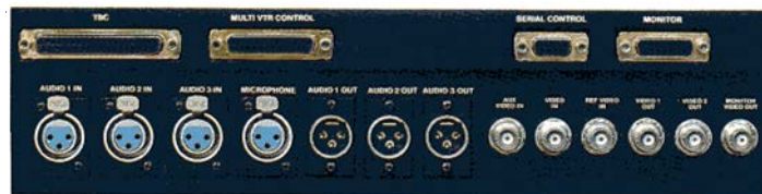
The rear I/O panel will accept all Ampex VPR accessories including remote controllers and monitoring.
